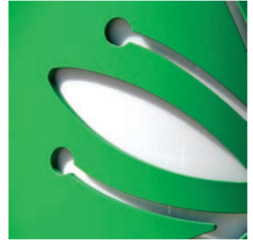
Detail of waterjet cut “wallflower” design
